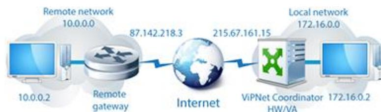
*Figure 3: Connecting over the IPsec protocol*
